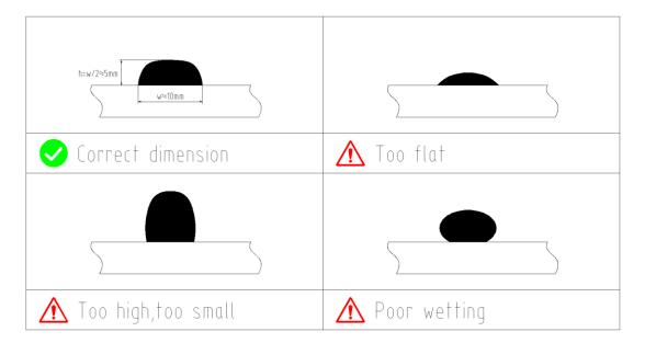
The correct form of structural adhesive after pasting modules
